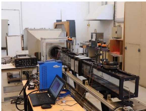
Fig. 3. (left) Aeroacoustic test bench; (right) aerosol spectrometer and particle size counting.
