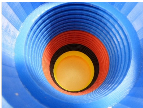
Fig. 1. (left) inner view of a 3D printed ABH and (right) its acoustical performance (bottom).
